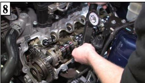
**8 Tighten Up:** The Comp Thumpr cams we're using are designed to work with the stock valvesprings, so they won't need to be replaced. These cams spec out to 226/246 duration at 0.050 lift. For installation, simply reverse the disassembly process, making sure to torque the cam caps (with oil on the threads) in stages until you get to 89 inch pounds. Begin with the center cap and work your way outward.
