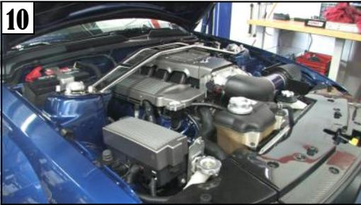
**Back Together:** Now repeat the process on the other side of the engine, and once you've finished bolt everything back up. Crank the engine and take a few moments to check for leaks and/or strange sounds. Having your engine professionally dyno tuned to take advantage of the more aggressive cams is also a good idea.
