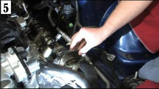
**5 Pull the Sprocket:** Remove the cam bolt that holds the timing sprocket and the cam phaser (in front of the sprocket) to the camshaft. You may have to wedge a small pry bar or large screwdriver behind the sprocket to help pull the sprocket off. If you can help it, don't remove the timing chain from the sprocket.
