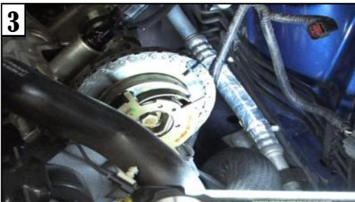
**Mark Your Spot:** To get the old cam out you will have to separate it from the timing gear, but before you do use a permanent marker to mark the position of both the chain and the timing sprocket. This will help you ensure the new cams are properly timed up on reassembly. The chains shouldn't have to come off, but this is good insurance.
