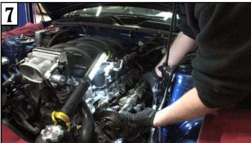
**7 De-cam:** Now you are ready to pull the stock cam right out. Make sure the camshaft housing bores in the head are clean then prepare them for the new cams by applying some assembly lube to them as well as the caps.
