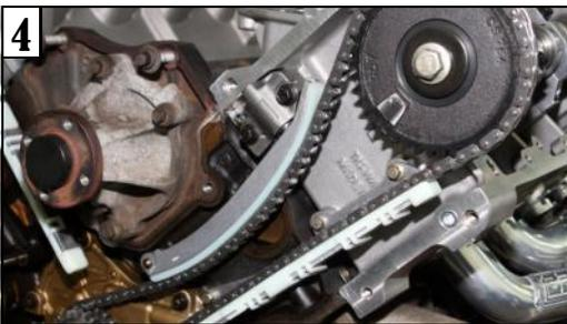
**Release the Tension:** The chain tensioners on each side will need to be pulled back enough to allow some slack in the timing chains so that the sprockets can be slid off the end of the cams. The tough way to do this is to remove the front cover to access the tensioners, but Ford sells a tool (it's actually just a nylon wedge on the end of a wire) that you can use to wedge between the tensioner and the chain without having to remove the front cover.
