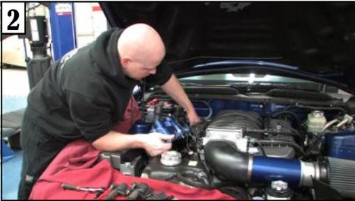
**Dig In:** If you are already familiar with Mustangs, this is an install that can be completed in an afternoon. The first step is to gain access to the camshafts. This will require removing any engine covers, wiring, disconnecting a few fuel lines, removing the coil packs and unbolting the cam covers.
