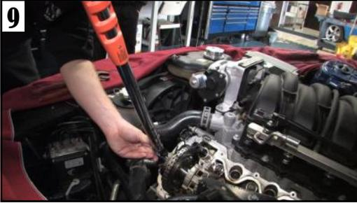
**Don't Recycle:** The stock bolt holding the cam phaser and timing sprocket to the camshaft is a torque-to-yield bolt and should not be reused. Purchase a new bolt from your local Ford dealer and install it to 30 ft/lbs and then turn it an additional 90 degrees.
